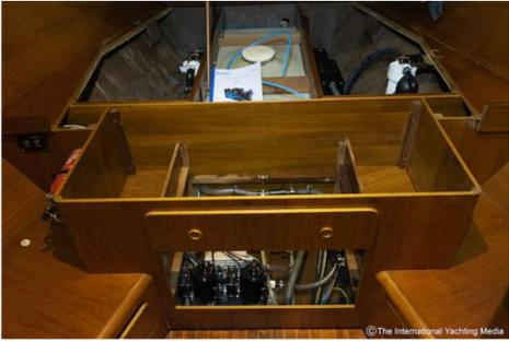
The **pump + filters group, in fact, is separated** from the machine body, which allows to install them almost everywhere. In our case, we installed the watermaker in the compartment below the bow bed!
